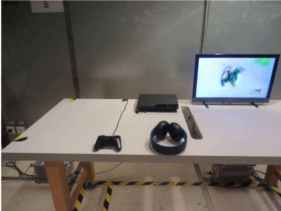
Test Setup Photo - Conducted Emission
