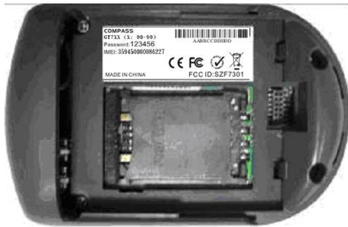
The FCC ID and DoC Label will be placed on the equipment as shown in the photograph below.
