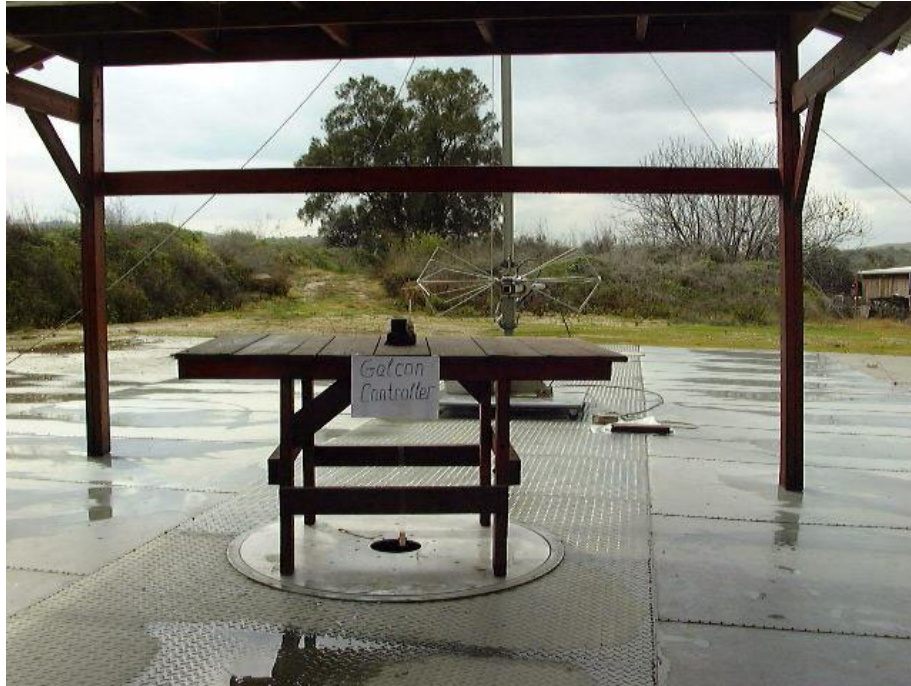
Figure 1. Radiated Emission Test
