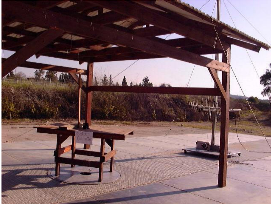
Figure 26. Radiated Emission Test. Front
