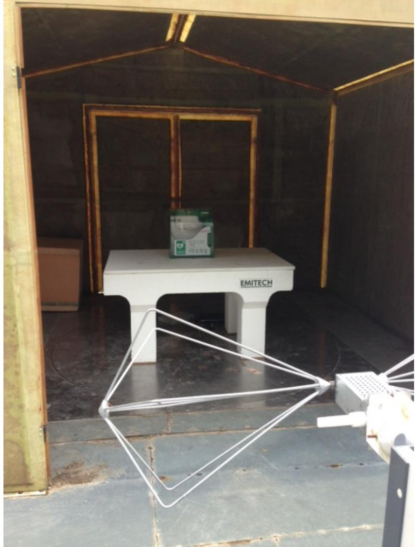
Radiated measurement on open area test site
