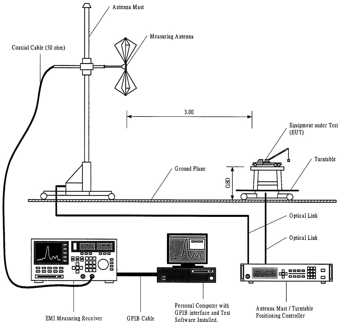
With hand-held or portable EUT exploratory radiated emission test shall be carried out, including rotation of the EUT through three orthogonal axes to determine the attitude that highest emission relative to the limit. The so found attitude and equipment arrangement shall be used in the final measurement.
