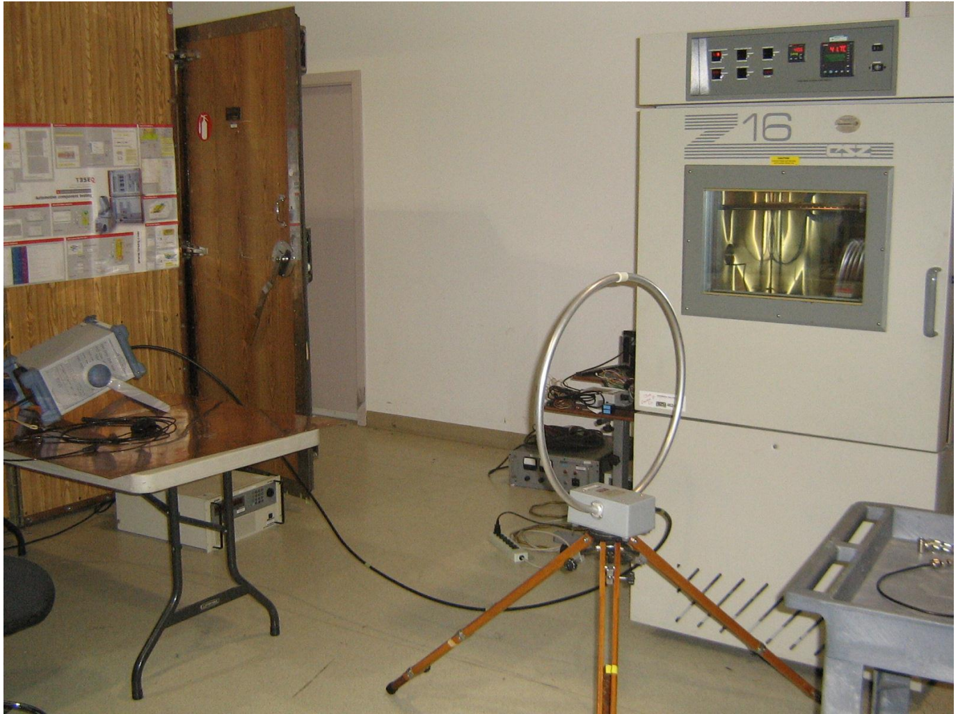
Frequency Stability Test in Environmental Chamber
