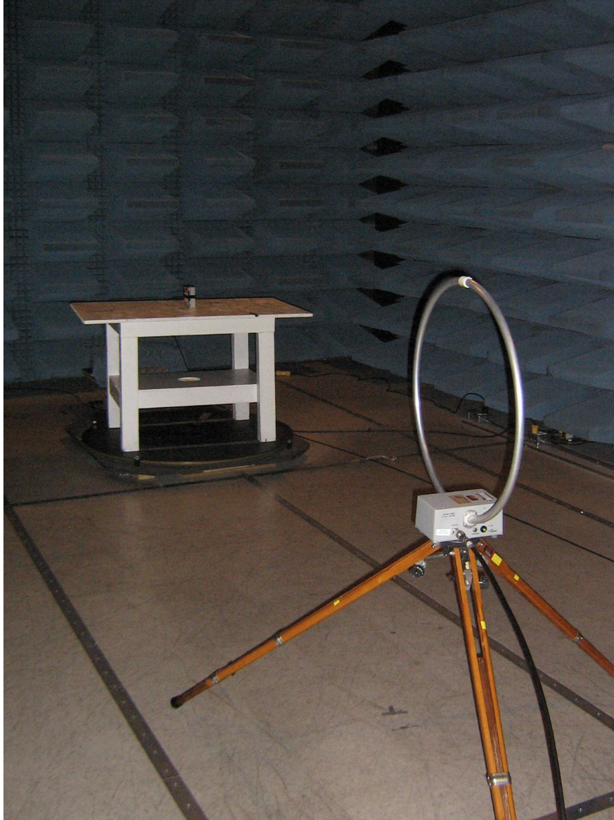
Radiated Emission Test Setup in the Semi-Anechoic Chamber
