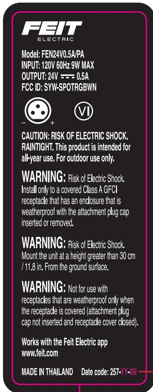
“257-YY-WW” is the factory date code: “257” means vendor number, “YY” means year of production, “WW” means week of production. above date code marked according to the actual production date.
