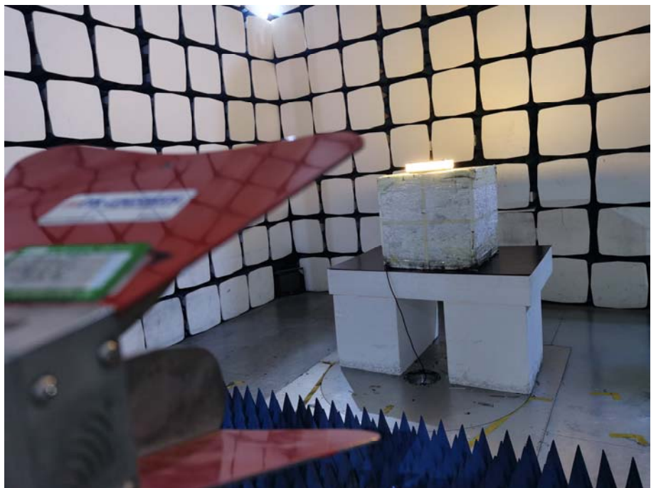
Radiation Emission Test Setup (1GHz to 18GHz)
