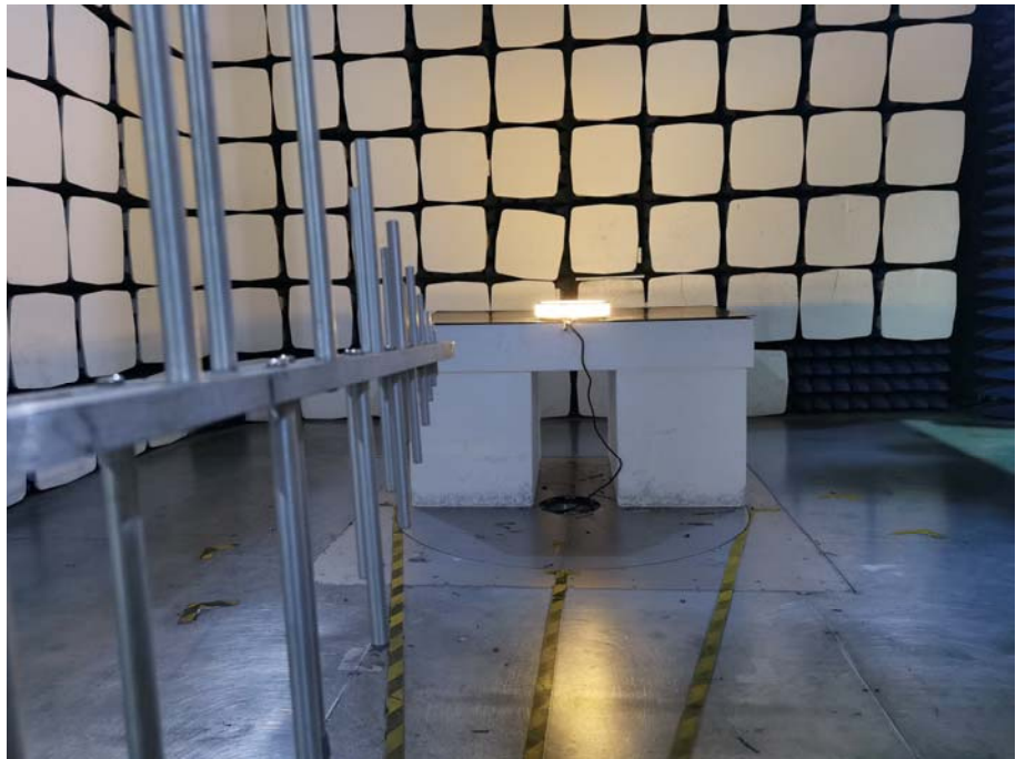
Radiation Emission Test Setup (30MHz to 1GHz)
