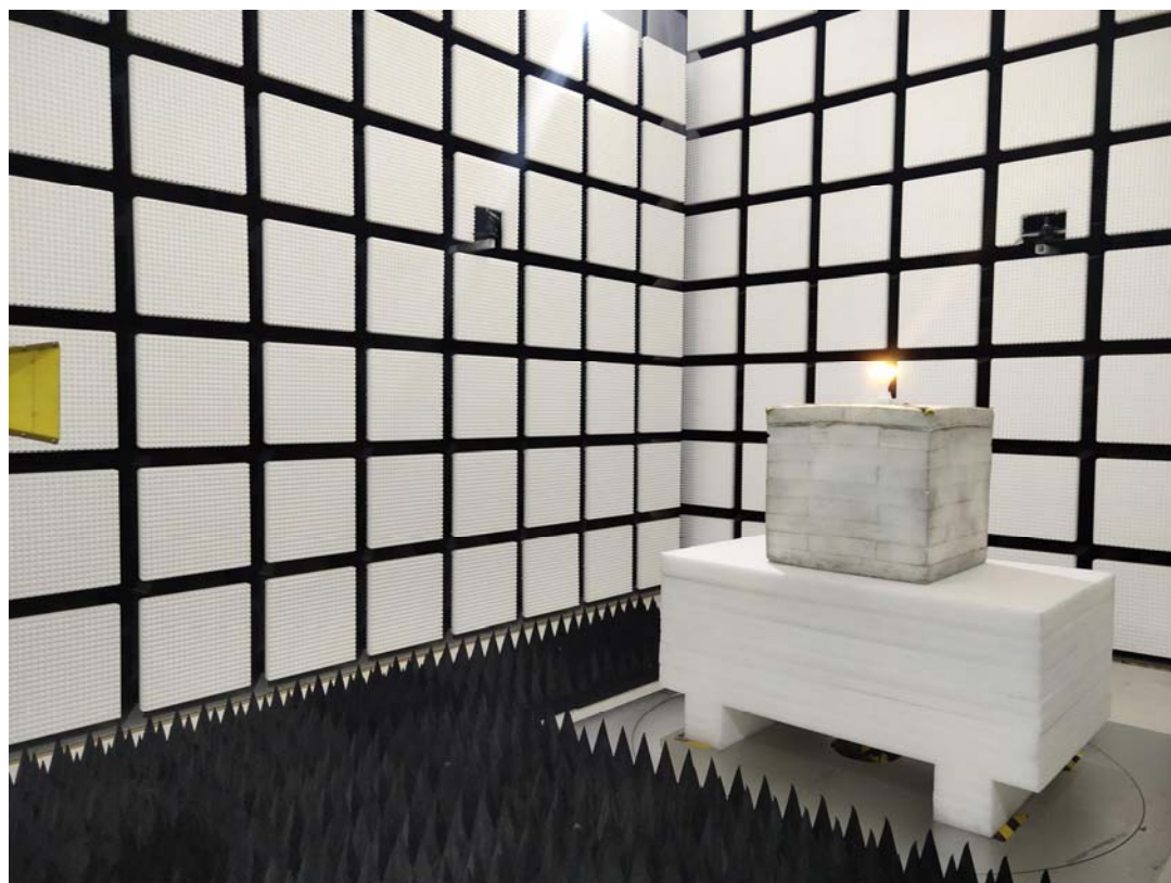
Radiated Emission Above 1GHz View
