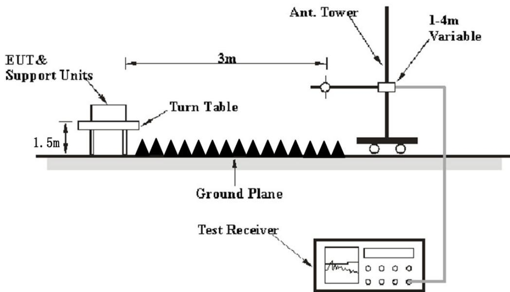
The radiated emission tests were performed in the 3 meters test site, using the setup accordance with the ANSI C63.10 - 2013. The specification used was the FCC 15 § 15.209, 15.205 and 15.231.
