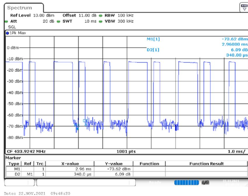
The graph shows the duration of 'on' signal. From Marker 1 to Delta 2, duration is 0.34ms.
