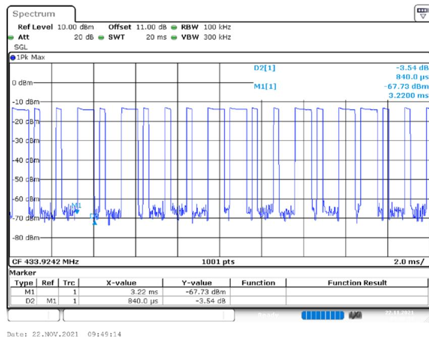
The graph shows the duration of 'on' signal. From Marker 1 to Delta 2, duration is 0.84ms.
