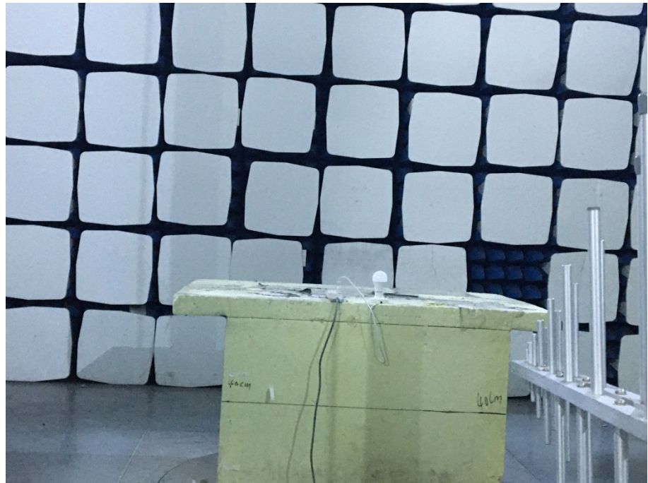
Radiation Emission Test Setup (30MHz to 1GHz)
