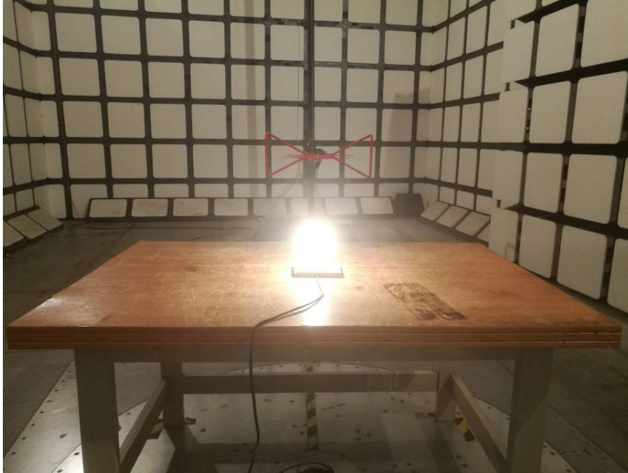
Radiated Emissions View (Below 1 GHz)
