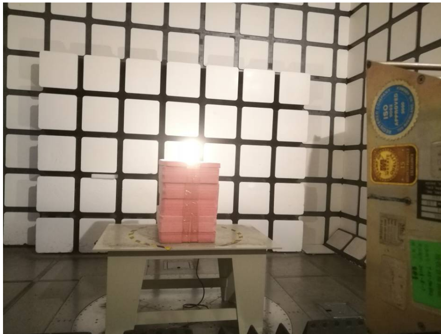
Radiated Emissions View (Above 1 GHz)
