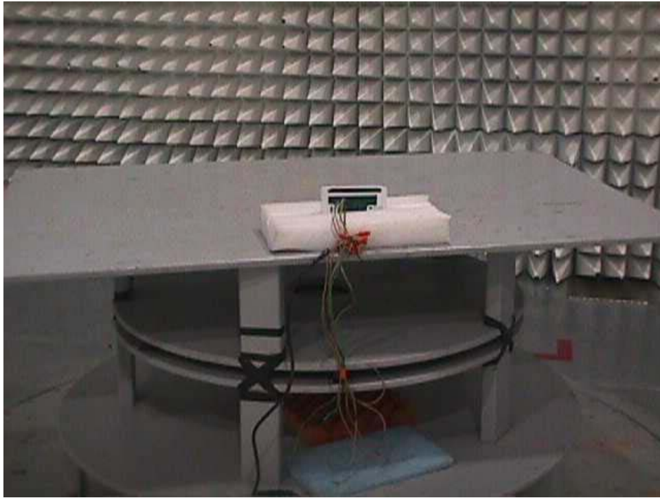
Radiated Emissions Test Configuration
