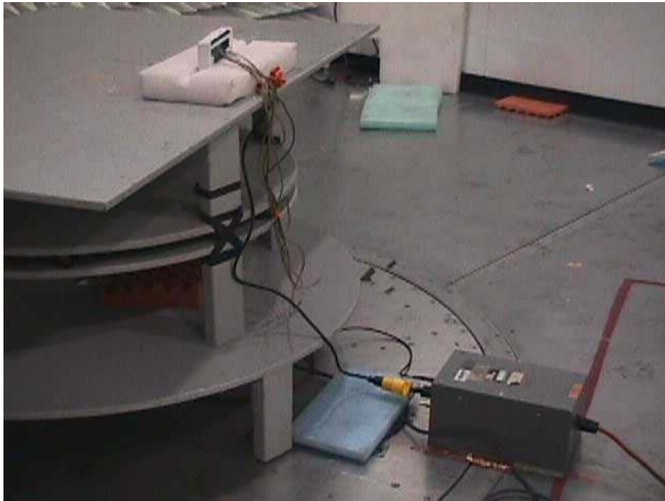
Line Conducted Emissions Test Configuration
