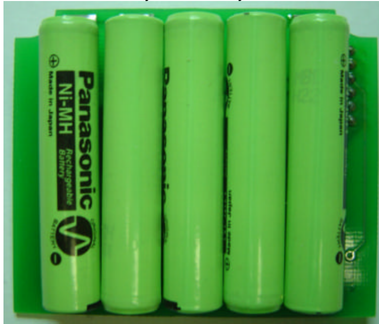
Battery Board-Battery Side
