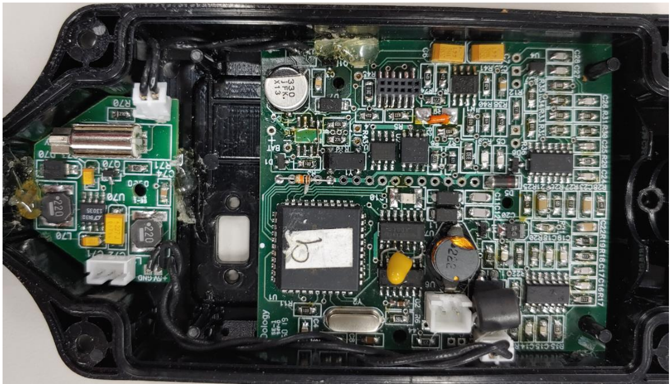
Main PCB installed
