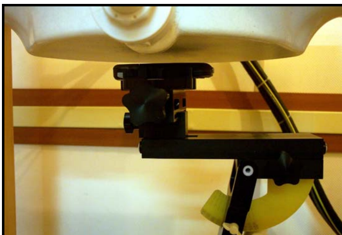
Figure 9.5 Muscle SAR Test Setup -- 15mm Distance Position --
