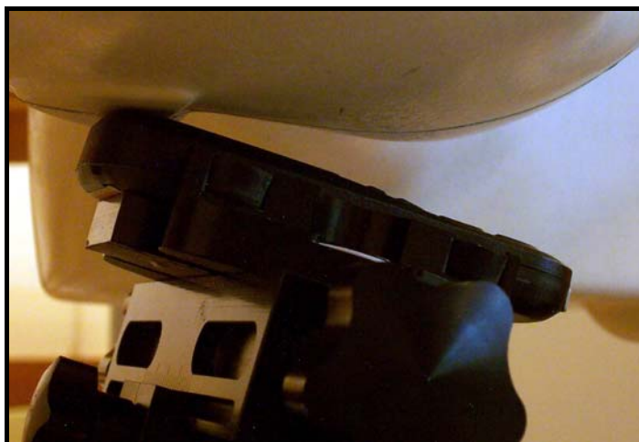
Figure 9.8 Right Head SAR Test Setup -- Ear / Tilted Position --
