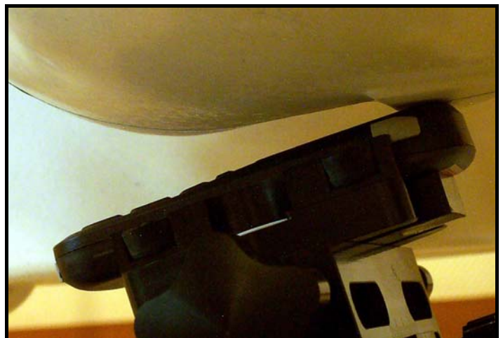
Figure 9.10 Left Head SAR Test Setup -- Ear / Tilted Position --
