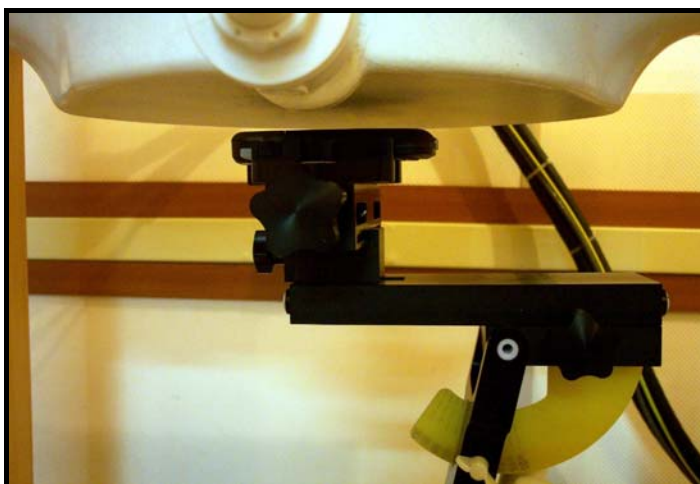
Figure 9.11 Muscle SAR Test Setup -- 15mm Distance Position --
