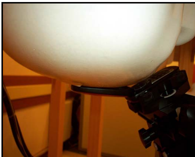
Figure 9.7 Right Head SAR Test Setup -- Cheek / Touch Position --
