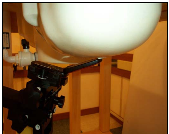
Figure 9.10 Left Head SAR Test Setup -- Ear / Tilted Position --
