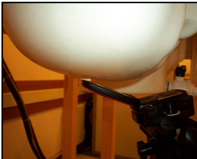
Figure 9.2 Right Head SAR Test Setup -- Ear / Tilted Position --
