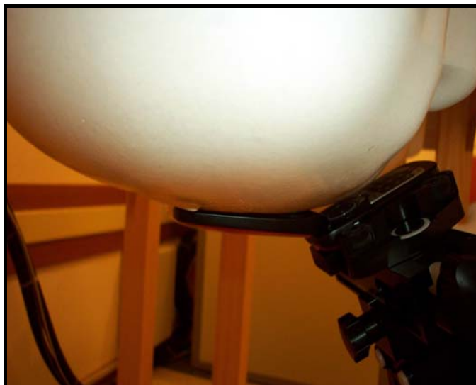
Figure 9.1 Right Head SAR Test Setup -- Cheek / Touch Position --
