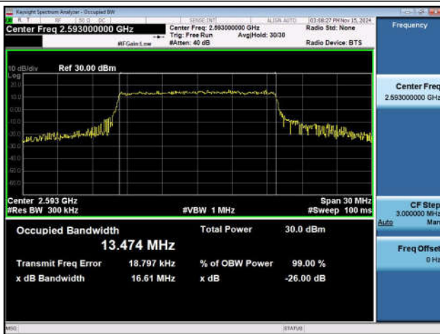
Band41-20MHz-QPSK-40620-100RB#0-PASS
