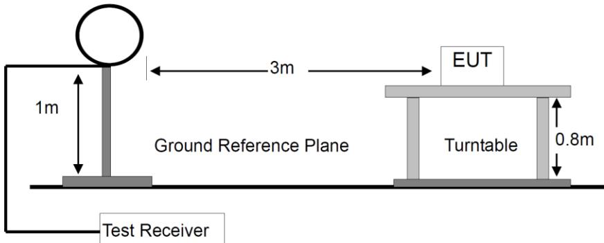
For Radiated Emission 30-1000MHz
