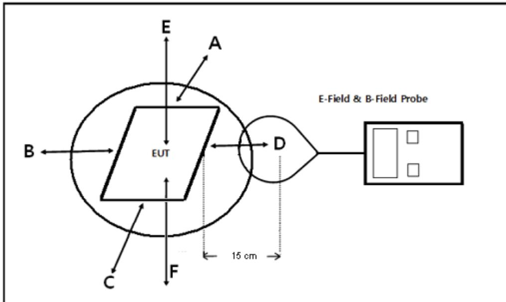
Note: As bottom point is not required to test for desktop devices, so we scanning all the surfaces and recorded the worst level in E.
