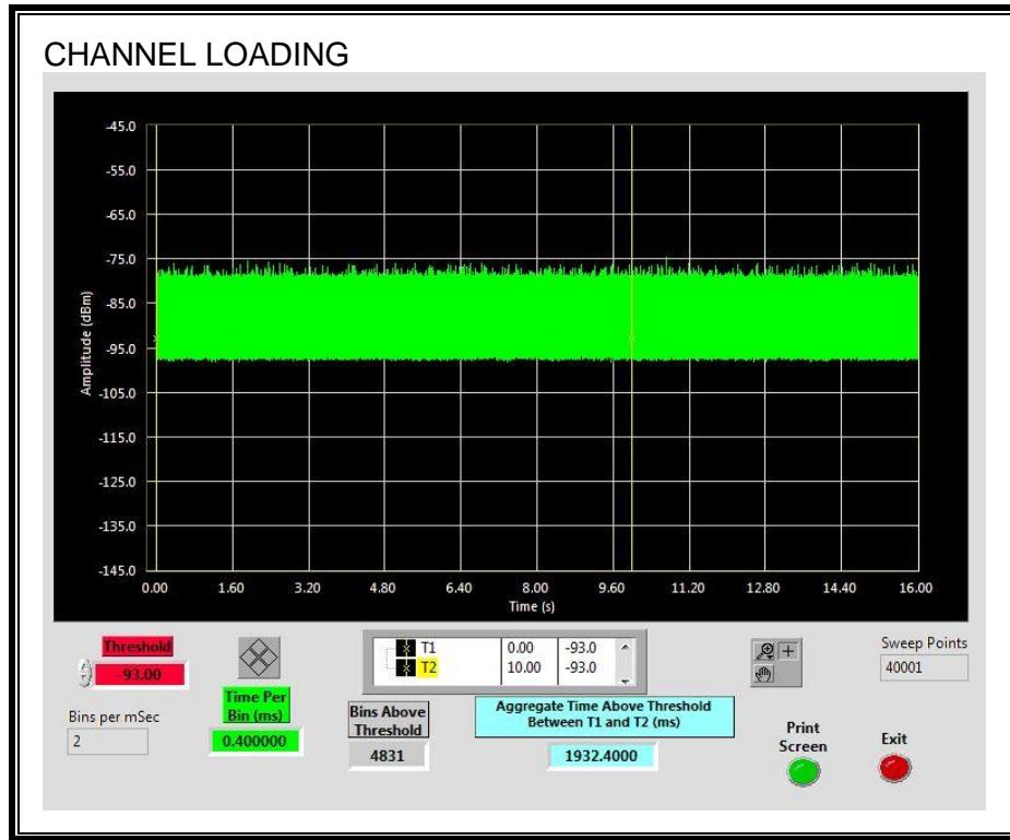
The level of traffic loading on the channel by the EUT is 19.32%
