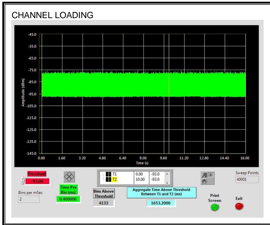
The level of traffic loading on the channel by the EUT is 16.53%
