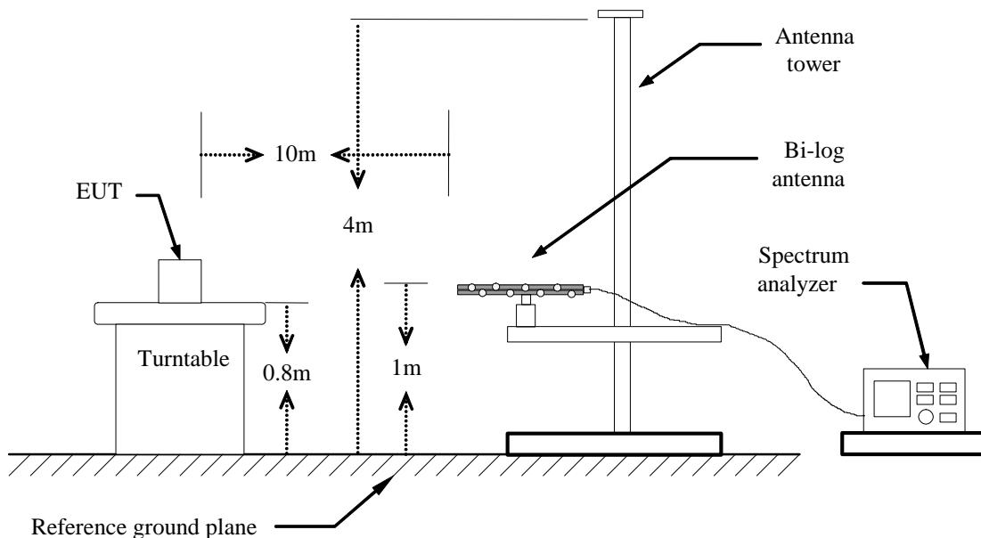
**Above 1 GHz**
