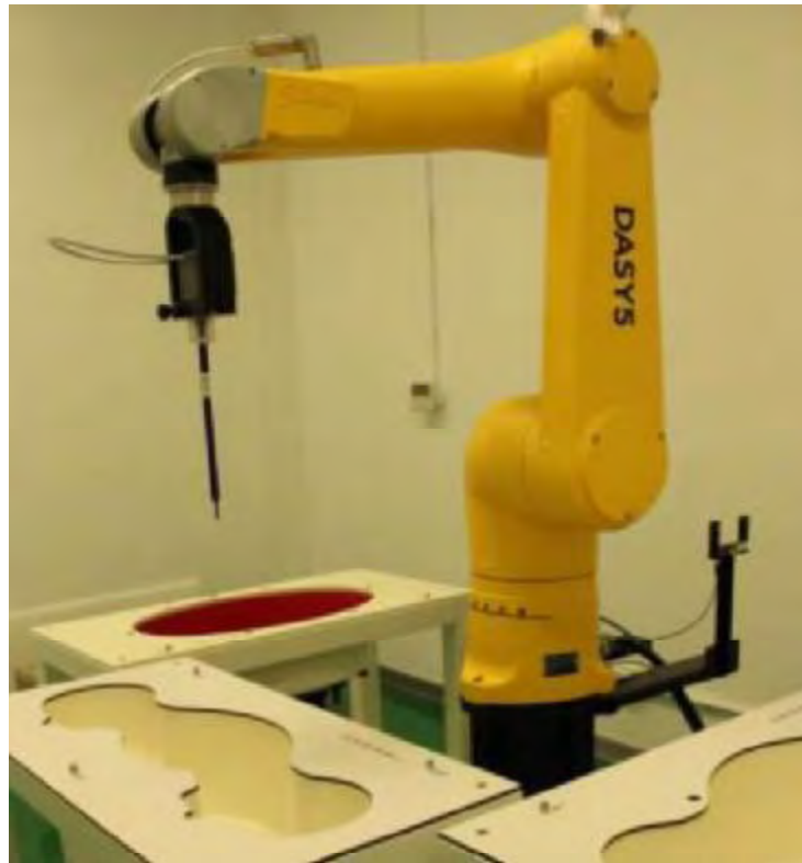
Picture 15-1: Specific Absorption Rate Test Layout
