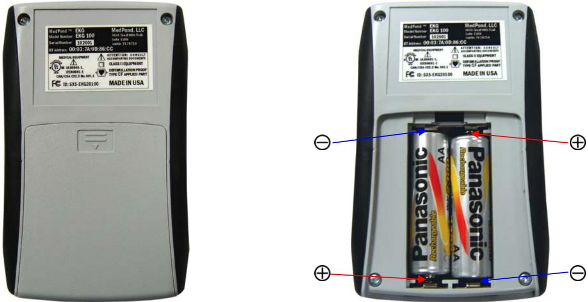
The battery cover slides down to expose the battery compartment. The battery used in the Ambulatory Cardiac Recorder device was selected to be a balance between long-life, light weight, and easy availability. Ambulatory Cardiac Recorder device uses standard 2 standard Ni-MH AA rechargeable batteries that are available in most drug stores, hardware stores, grocery stores, or on the Internet.
