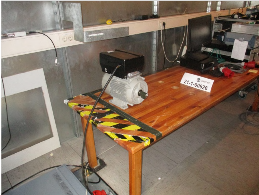
Photograph 1: Mains conducted emission measurements test set-up
