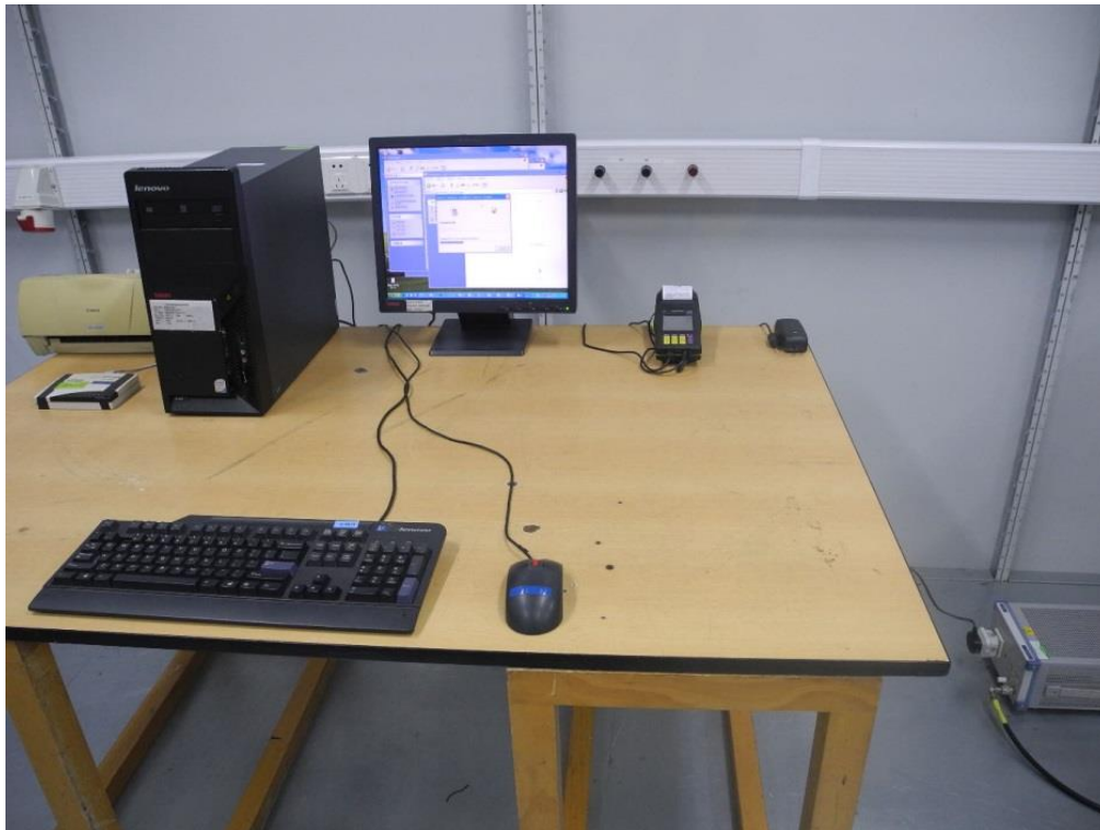
AC Conducted Emission Test Setup Front
