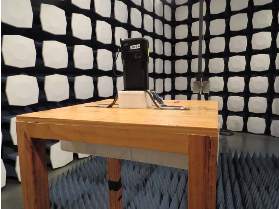
Picture 2: Radiated Spurious Emissions Test setup
