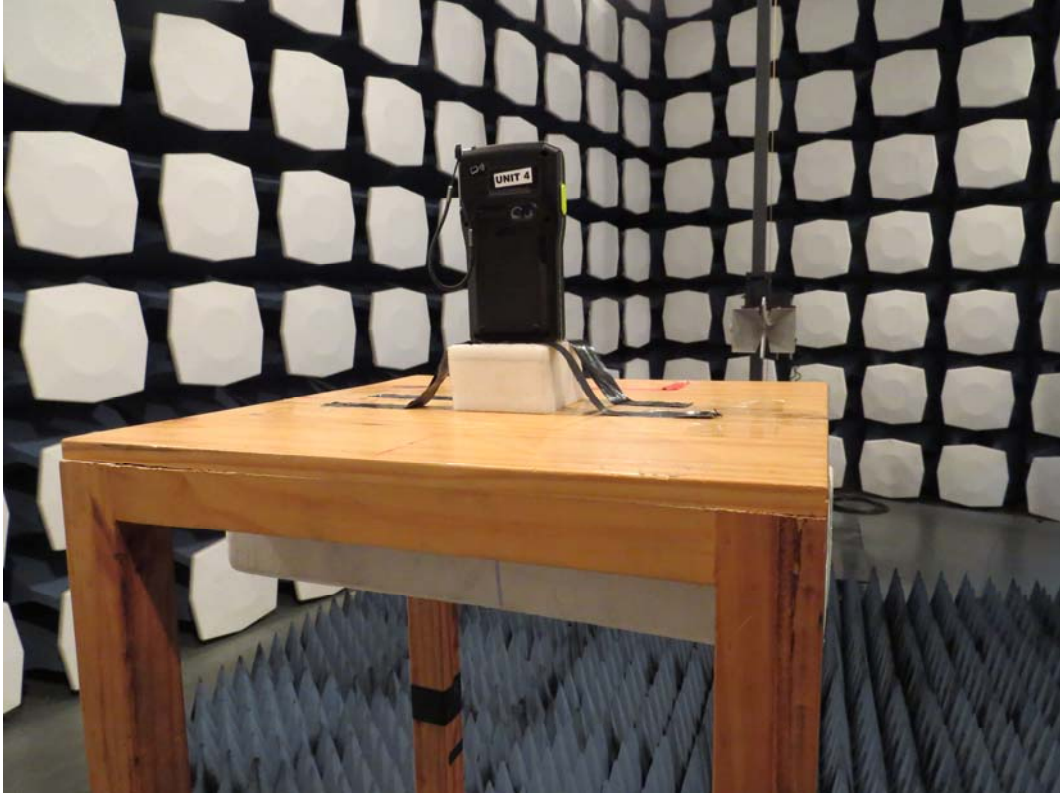
Picture 2: Radiated Spurious Emissions Test setup
