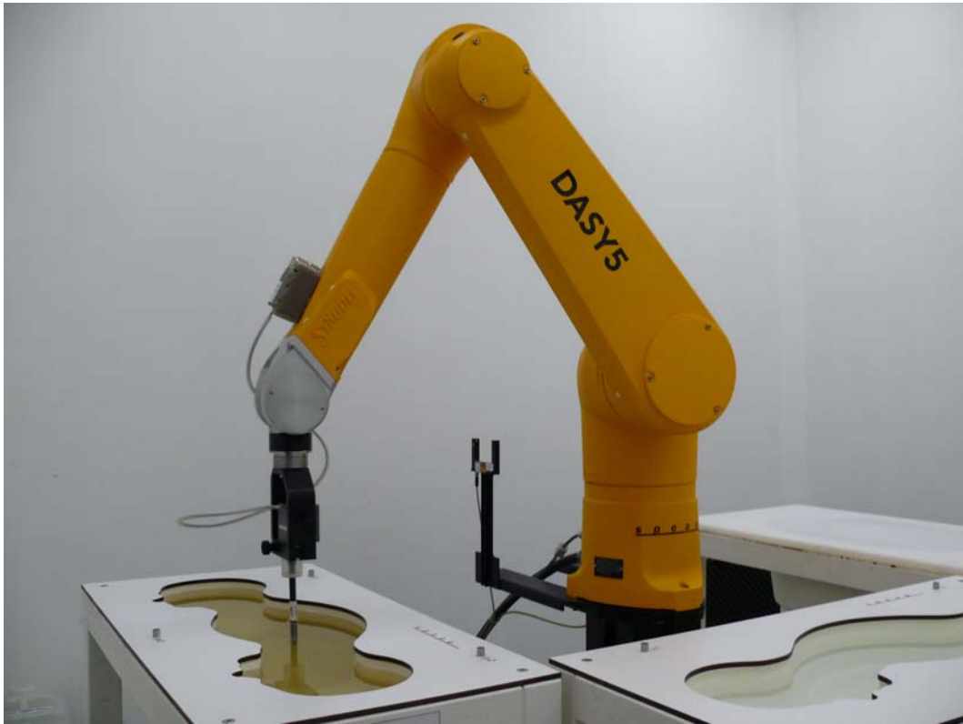
Picture 1: Specific Absorption Rate Test Layout
