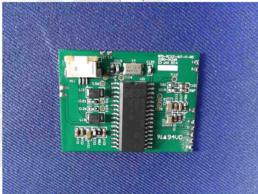
Figure 18 PCB of the EUT-Module View (RFID)
