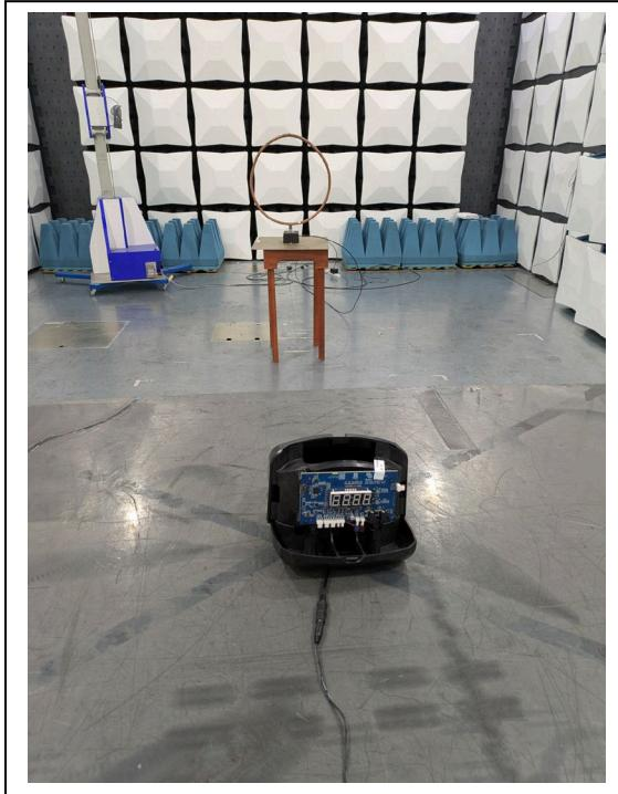
**Radiated Spurious Emission: 30 MHz to 1000 MHz**
