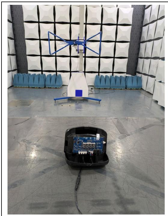
**Radiated Spurious Emission: 1 GHz to 18 GHz**
