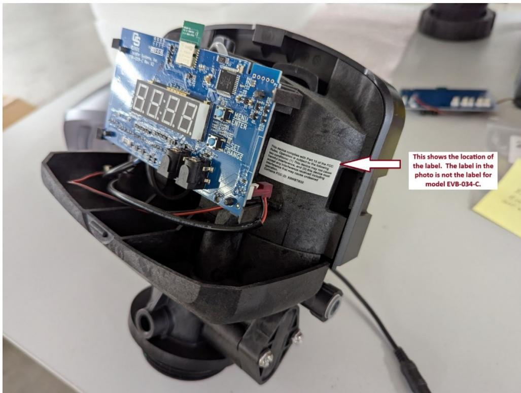
The selected location is in a conspicuous location under the main slide cover of the valve. The cover is easily removed without tools and this is the same area that a user would access to manually change settings using the user interface, or to change the 9V backup battery. This location will protect the label from the elements while still making it noticeable to the end user.
