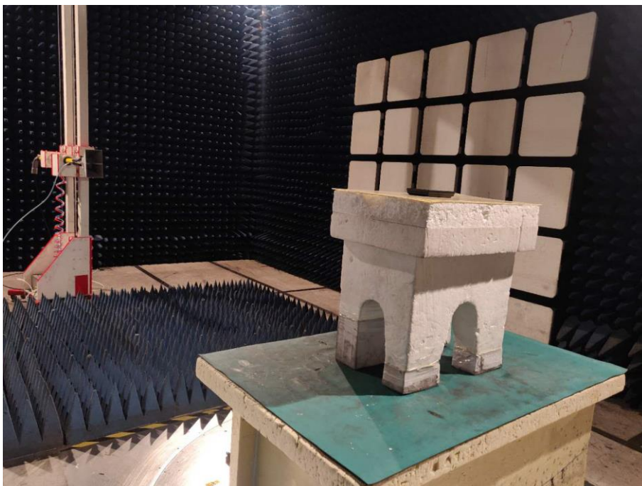
Spurious Emission Test Setup (Above 1GHz)
