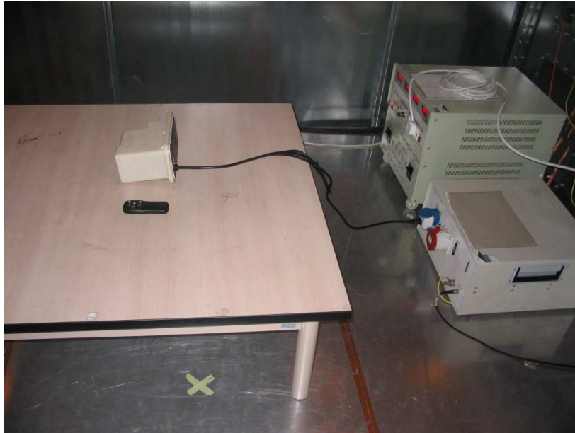
Photograph 1: Set-up for conducted emissions
