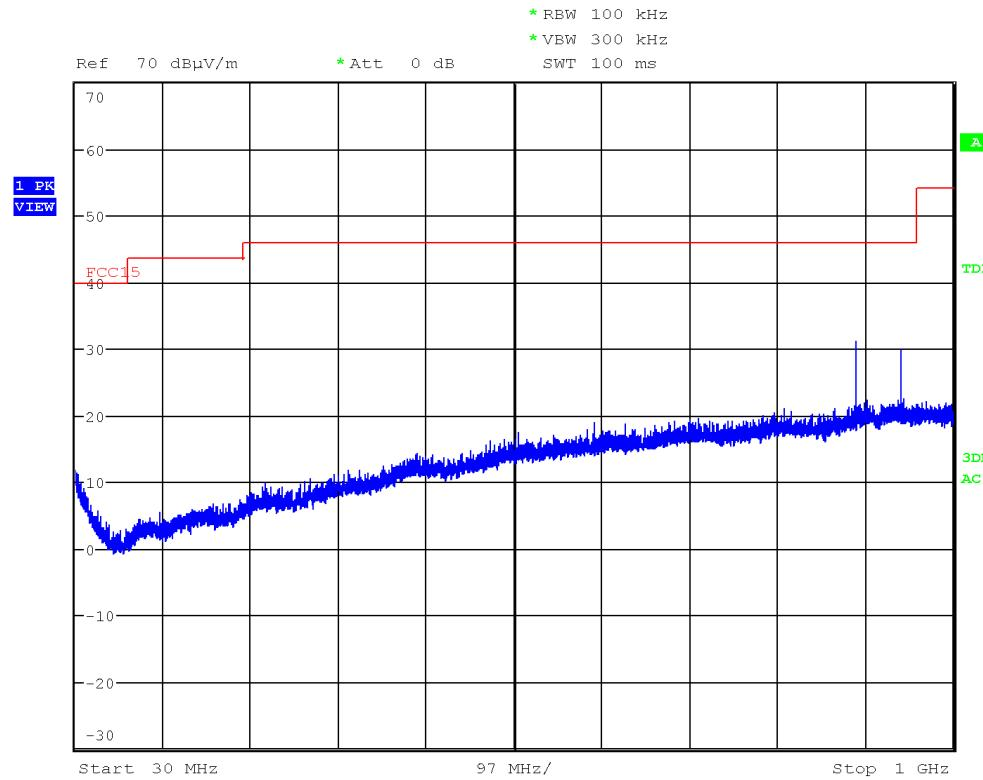
Note: The carrier was attenuated using a Notch filter.
