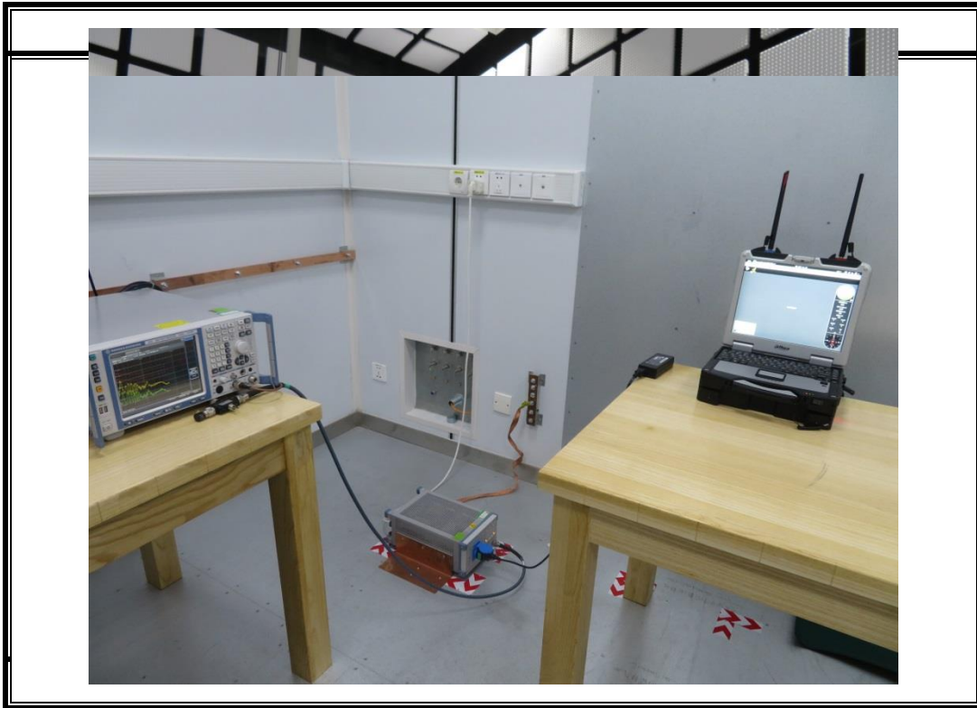
POWERLINE CONDUCTED EMISSIONS MEASUREMENT SETUP RADIATED RF MEASUREMENT SETUP (Below 30MHz)
