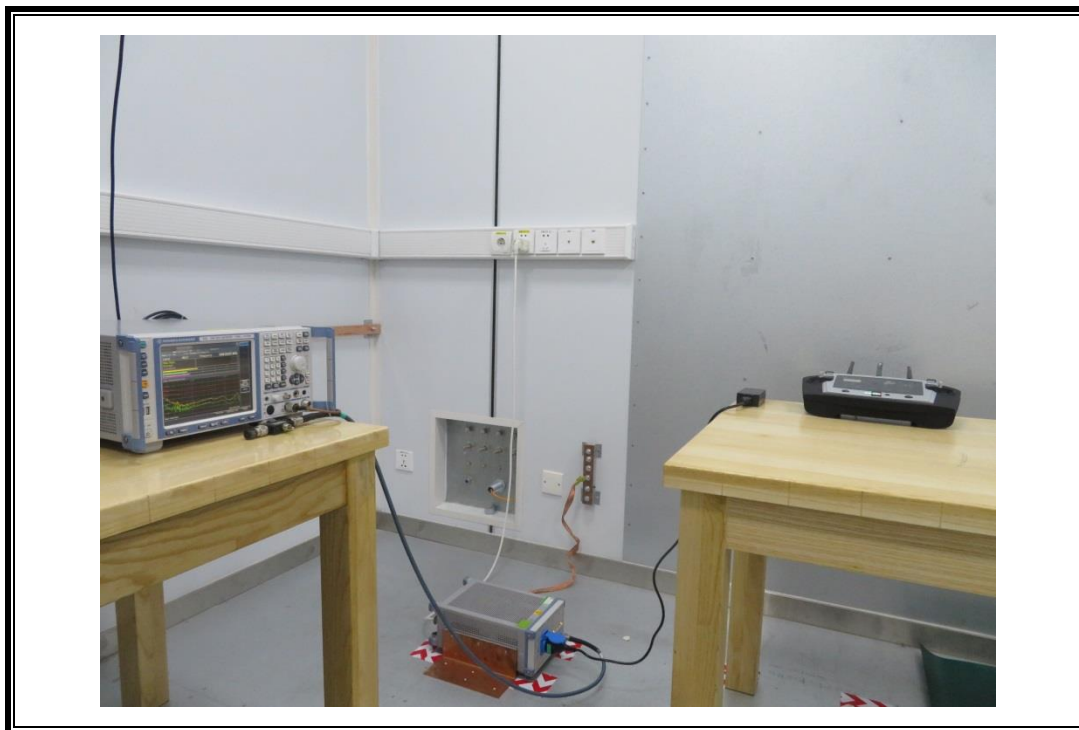
RADIATED RF MEASUREMENT SETUP (Below 30MHz)
