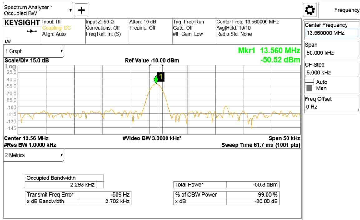
Remark: Because the measured signal is CW or CW-like adjusting the RBW per C63.10 would not be practical since measured bandwidth will always follow the RBW and the result will be approximately twice the RBW.
