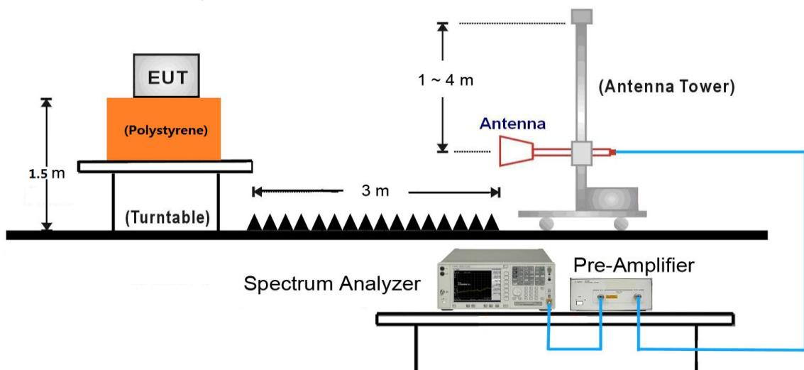
18GHz ~25GHz Test Setup:
