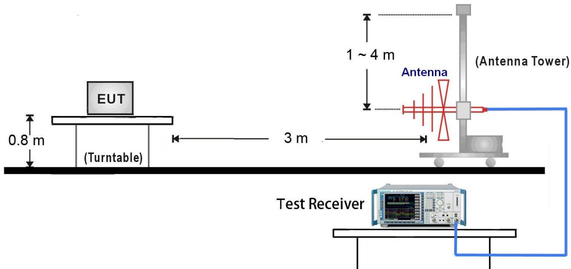
1GHz ~ 18GHz Test Setup:
