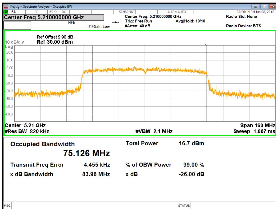
Note: Because 99% OBW for all channels and bandwidths are stays completely within the 5150-5250MHz band, so DFS test is not required.
