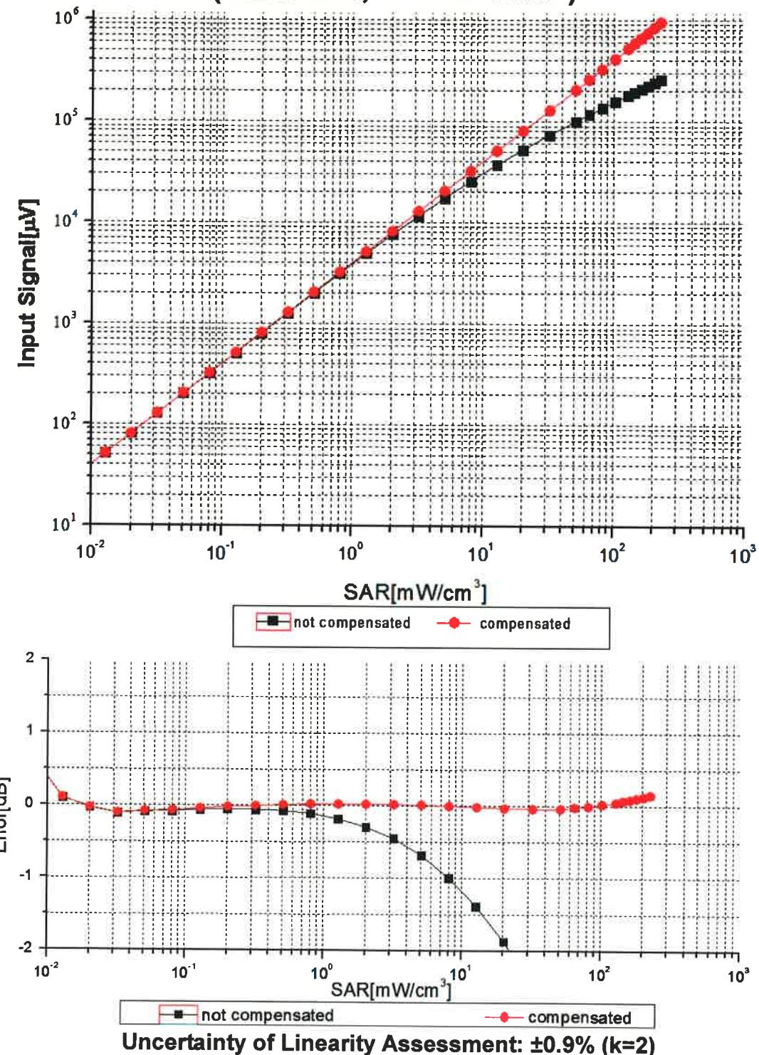
Note: Increased noise level was detected on Z-channel. This probe is not standard conform for SAR compliance testing if a DUT produces peak spatial SAR value smaller than 0.04 W/kg.
