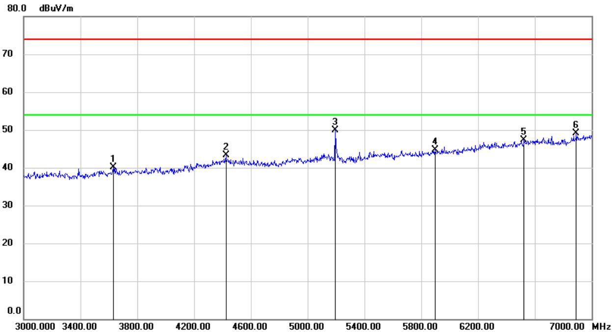
Note: 1. Measurement = Reading Level + Correct Factor.
