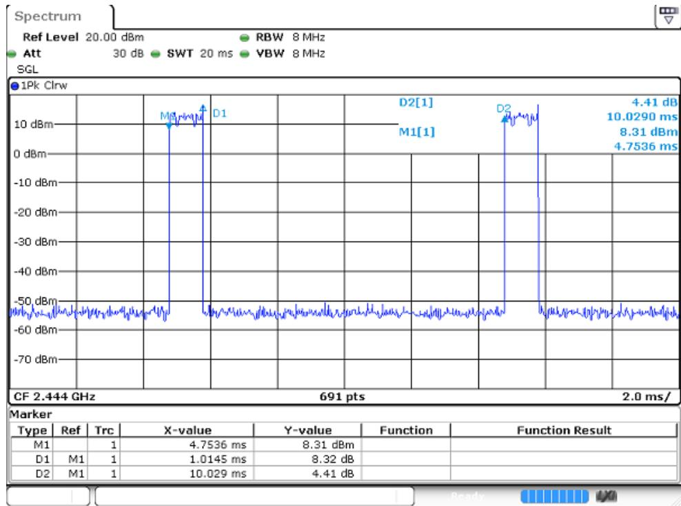
Note: The duty cycle of all modulations and bandwidths are the same, so we only report one mode and this will apply for all other mode.
