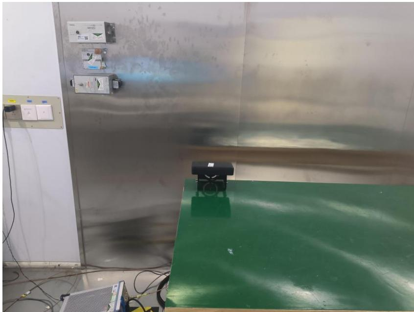
RF Radiated Test(30MHz-1GHz)
