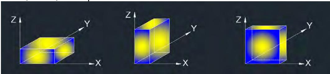
Note 1: For all radiated test, EUT in each of three orthogonal axis emissions had been tested, but only the worst case (Z axis) data recorded in the report
