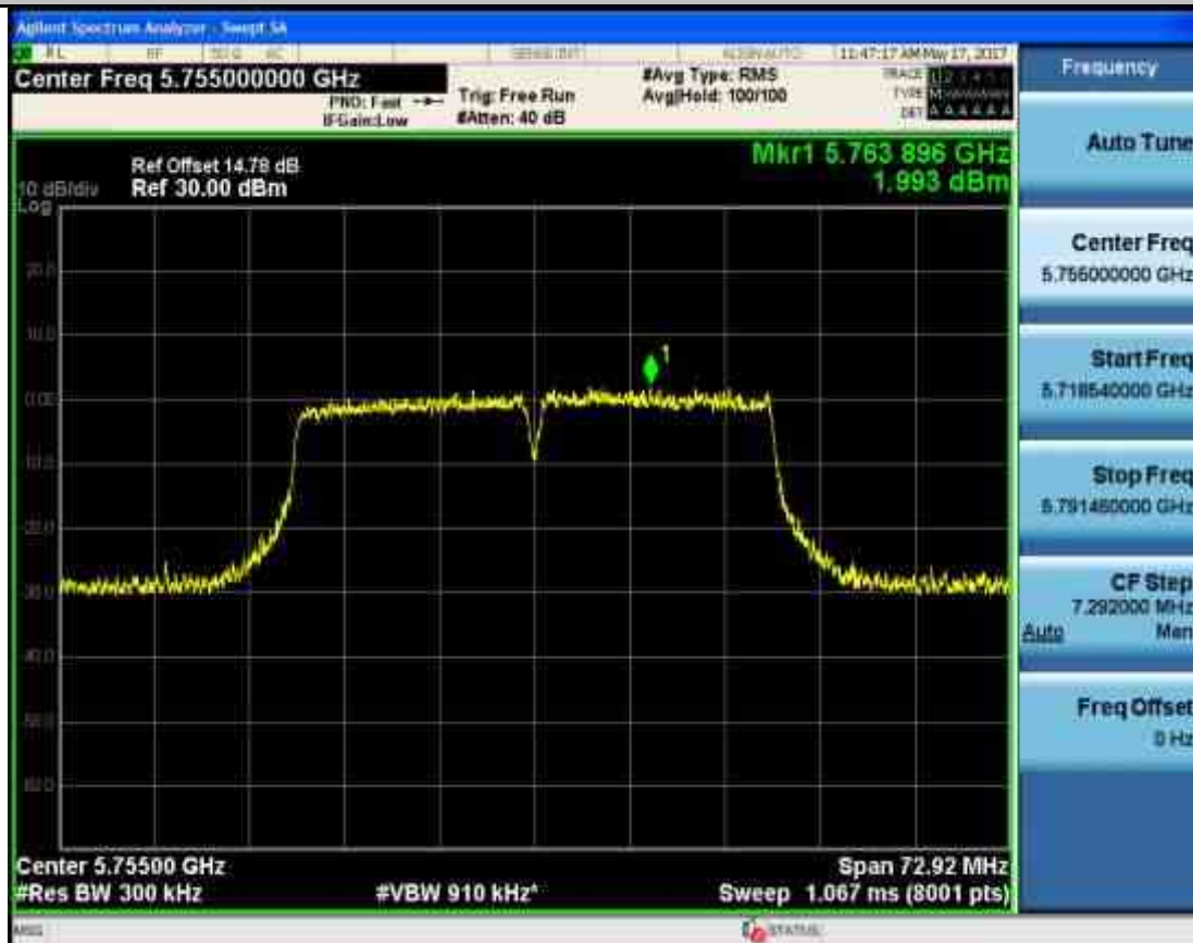
Maximum Conduct Output Power_TNVN_11N40MIMO_5795_Ant2
