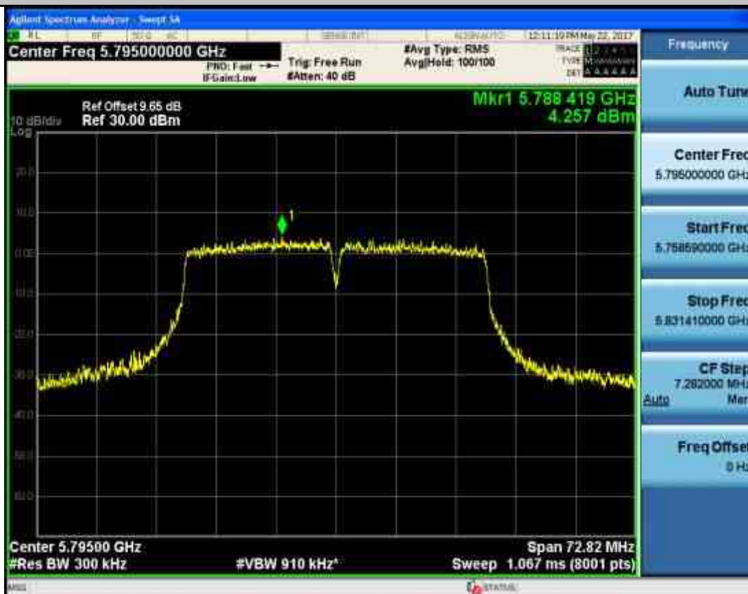
Maximum Conduct Output Power_TNVN_11AC80MIMO_5775_Ant1
