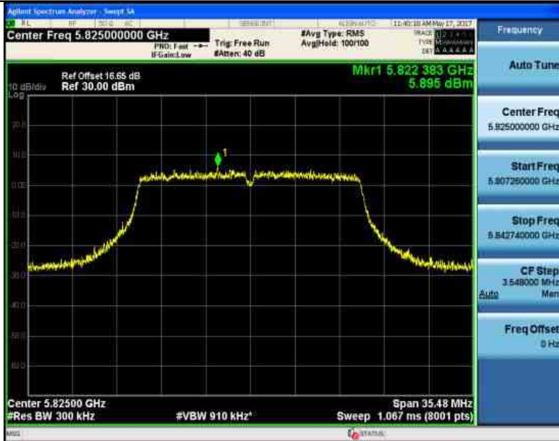
Maximum Conduct Output Power_TNVN_11N40MIMO_5755_Ant2
