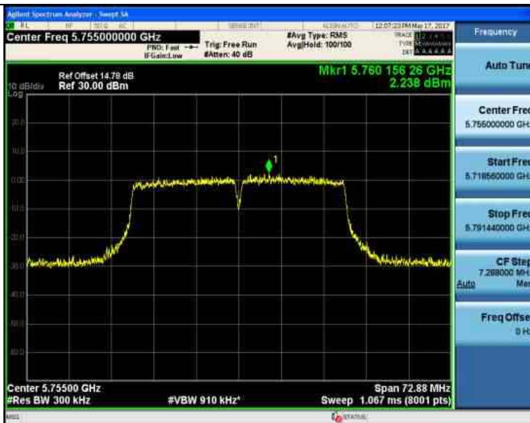
Maximum Conduct Output Power_TNVN_11AC40MIMO_5795_Ant2
