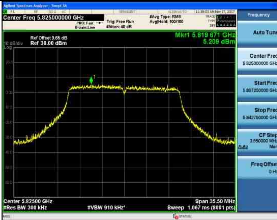
Maximum Conduct Output Power_TNVN_11N40MIMO_5755_Ant1
