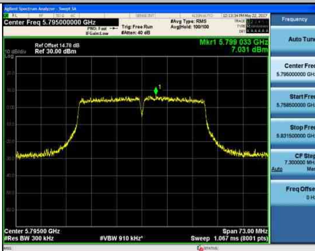
Maximum Conduct Output Power_TNVN_11AC80MIMO_5775_Ant2
