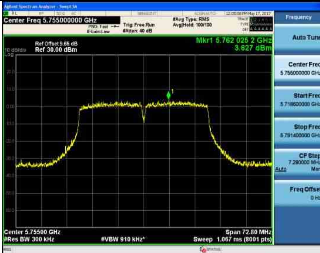
Maximum Conduct Output Power_TNVN_11AC40MIMO_5795_Ant1
