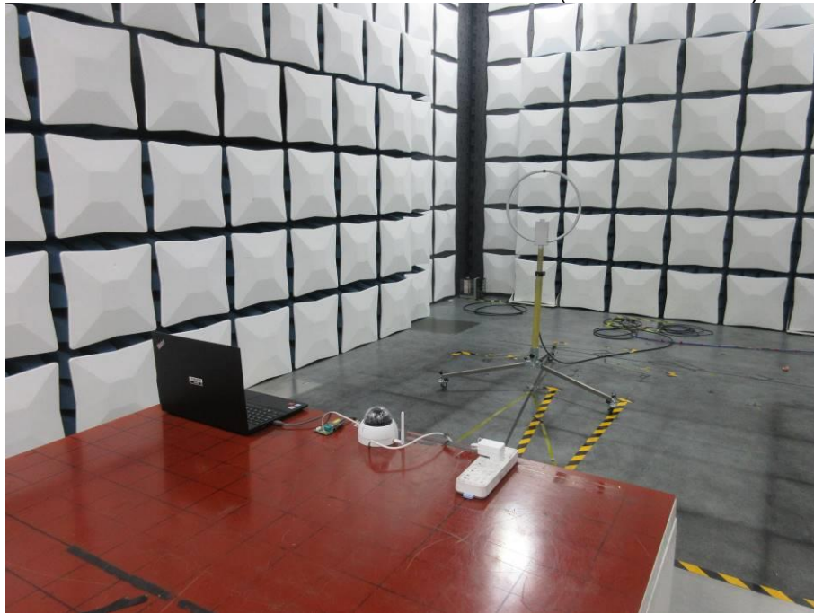
RADIATED RF MEASUREMENT SETUP (9KHz ~ 30 MHz)
