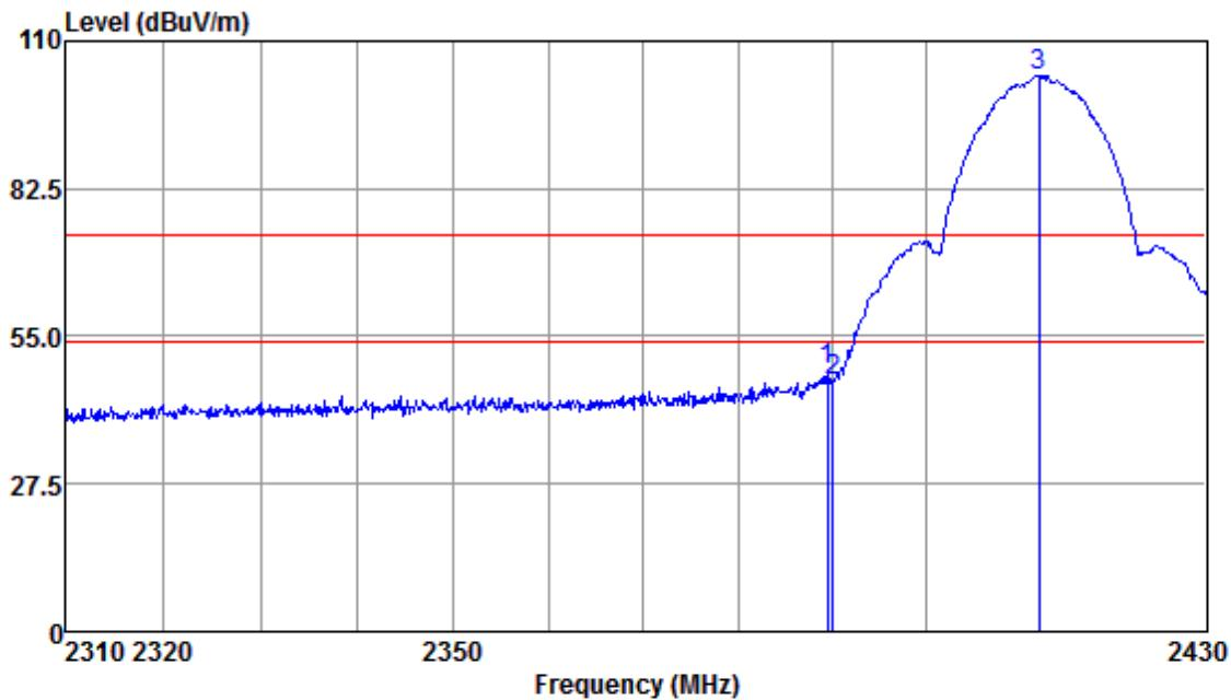
Mode:b; Polarization:Horizontal; Modulation:b; bandwidth:20MHz; Channel:High
