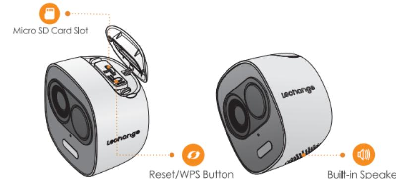
**Note:** The top cap can be opened with the pry bar from the accessory kit.
