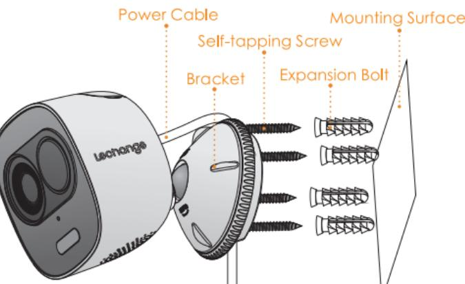
**Step 1** Drill screw holes on the mounting surface as the installation position map shows and put in the expansion bolts.
