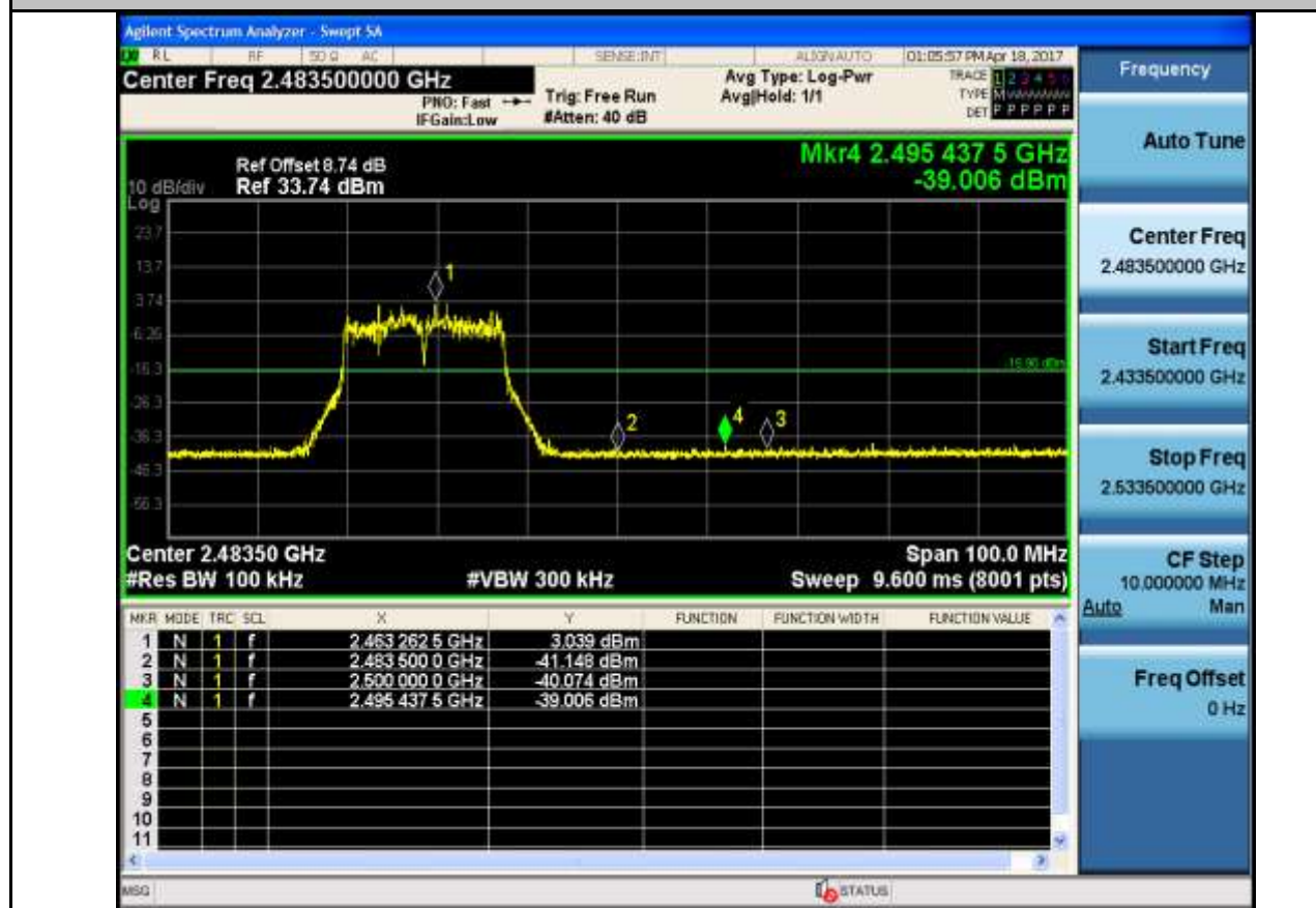
Band-edge for RF Conducted Emissions_11N40SISO_2422_Hopping Off
